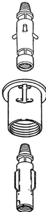
The "Top Drive" SIM-CAS system allows simultaneous drilling and casing by the casing being rotated whilst it follows the eccentric bit.
